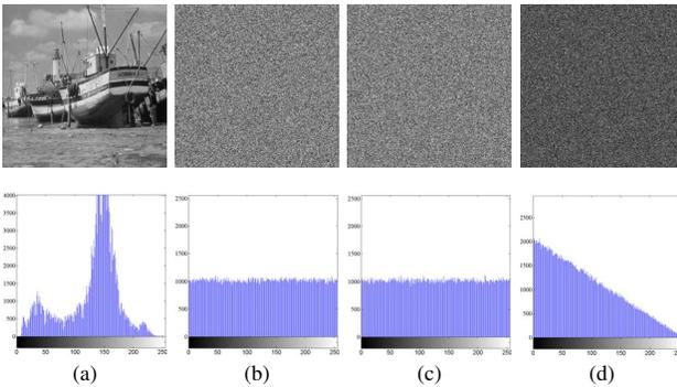
Fig. 6: Encryption key sensitivity analysis. (a) The original image  $P$ ; (b) the encrypted result  $C_1 = Enck(P, K_{e1})$ ; (c) the encrypted result  $C_2 = Enck(P, K_{e2})$ ; (d) the difference between  $C_1$  and  $C_2$ ,  $|C_1 - C_2|$ .
