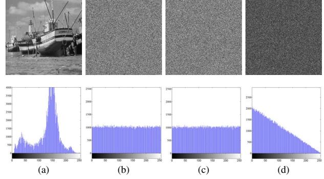
Fig. 7: Decryption key sensitivity analysis. The used ciphertext image  $C_1$  is from Fig. 6(a). (a) The decrypted image  $D_1 = Deck(C_1, K_{d1})$ ; (b) the decrypted image  $D_2 = Deck(C_1, K_{d2})$ ; (c) the decrypted image  $C_3 = Deck(C_1, K_{d3})$ ; (d) the difference between  $D_2$  and  $D_3$ ,  $|D_2 - D_3|$ .
