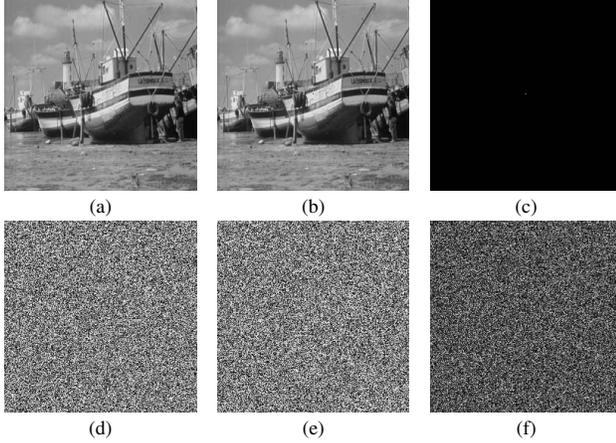
Fig. 8: Differential attack analysis. (a) The original image  $P_1$ ; (b) an image  $P_2$  generated by randomly changing one pixel of  $P_1$ ; (c) the difference between (a) and (b); (d) the encrypted result  $C_1 = \text{Enck}(P_1, K_e)$ ; (e) the encrypted result  $C_2 = \text{Enck}(P_2, K_e)$ ; (f) the difference between  $C_1$  and  $C_2$ ,  $|C_1 - C_2|$ .
