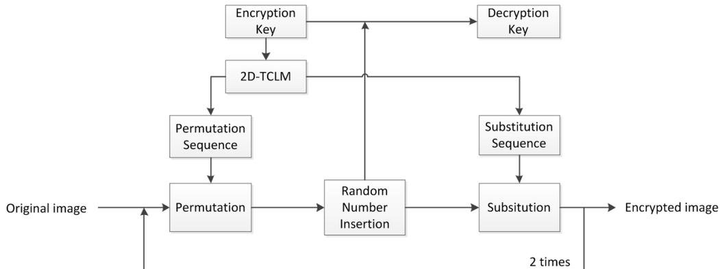
Fig. 2: The structure of proposed image encryption algorithm.
