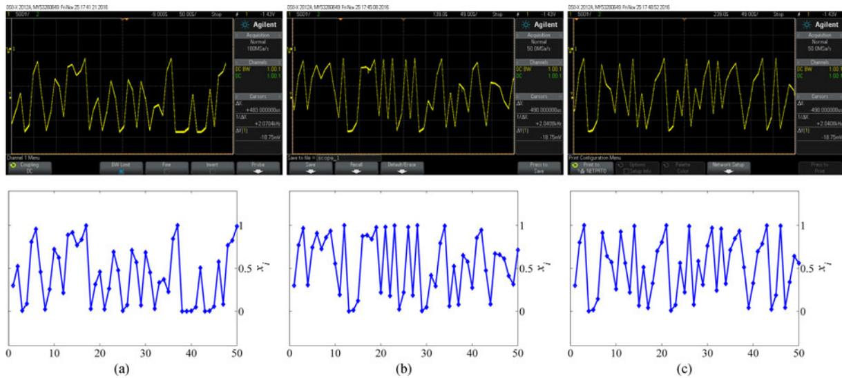
**Fig. 11.** Outputs of FPGA and MATLAB implementations of new chaotic maps. The top and bottom rows plot the first 50 iteration values of the (a) LS map, (b) LT map, and (c) TS map in the FPGA and MATLAB simulations, respectively. The initial states  $(x_0, r)$  are set as  $(0.3, 0.5)$  (namely  $(3FD3333333333333, 3FE0000000000000)$  in FPGA simulations).
