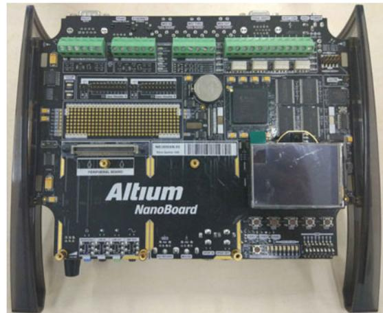
Fig. 10. Experimental realization of FPGA design.
